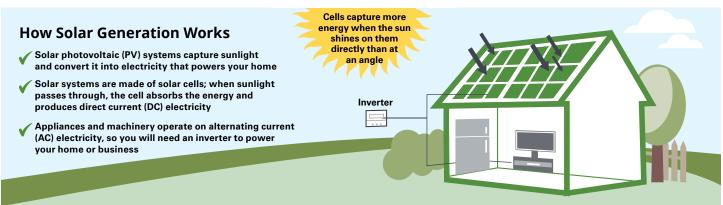
When you go solar, you are still connected to the SCE utility grid, so you can still receive power at night and other times when your solar energy system's output is lower. For solar only installations, if the power goes out in your area, your property will be affected as well.
